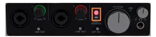
Talk into the microphone, ensuring there is a green light flashing when you speak. If this is not flashing, please increase the microphone level until the light flashes green. If the light is flashing red, please decrease the microphone level until the light flashes green.
